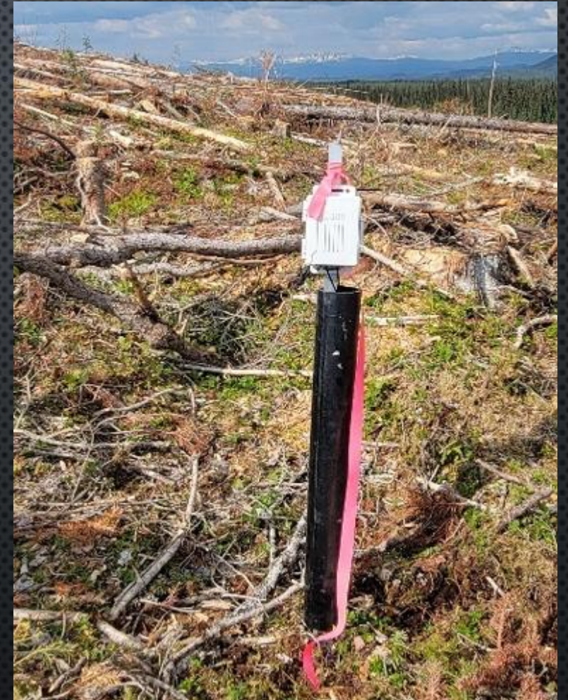
Soil moisture station: H21 data logger, 2 – 4 EC5 sensors, cables buried
