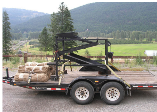
Plate 47. Custom cone cleaner fabricated using operational designs already in existence plus modifications to improve function.
