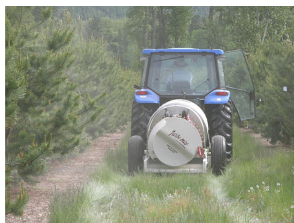
Plate 49. Sprayer in action creating ideal air flow conditions to assist fertilization of receptive female conelets.
