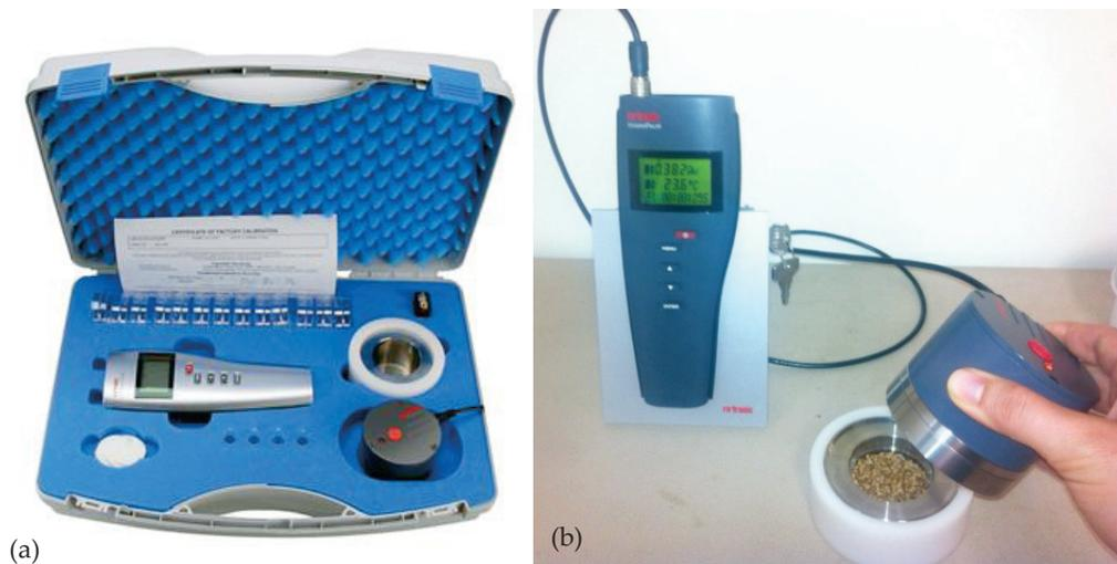
Figure 1. The Portable water activity meter (a) packed for transport and (b) in use at the BC Tree Seed Centre.
