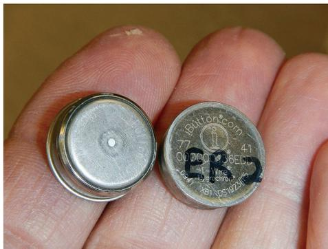
Figure 2. iButtons showing the relative humidity (RH) monitoring hole.
